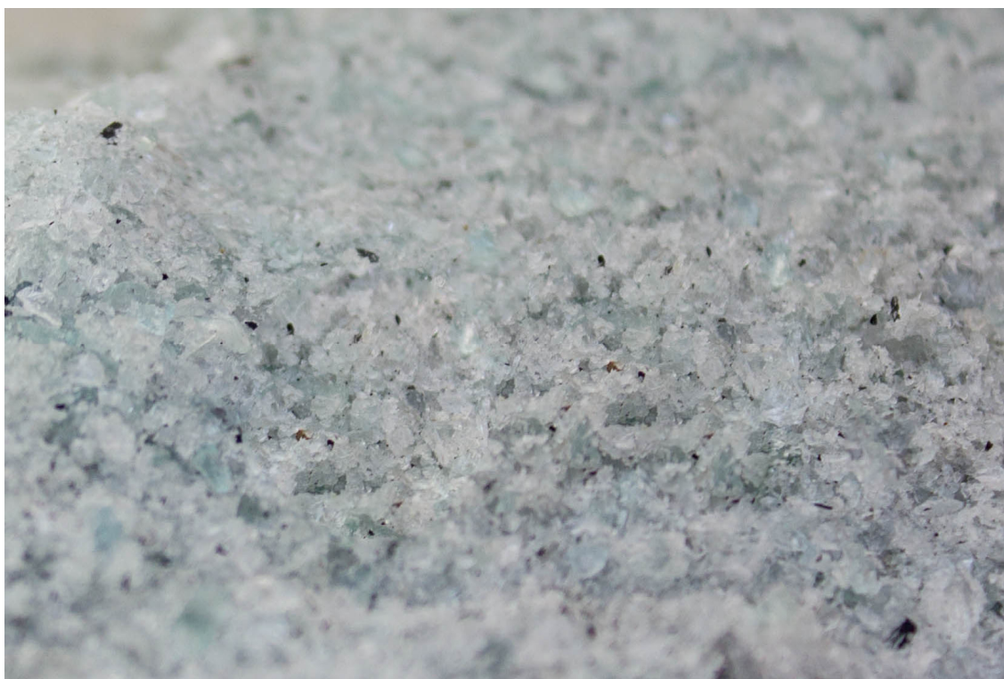
Figure 5 Selected sample of glass cullets. Granulation between 1-3 mm
