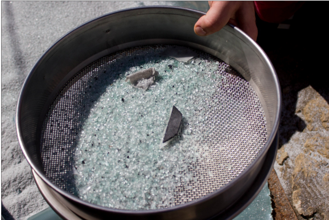
Figure 6 Testing with laboratory test sieve
